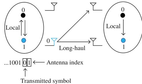
Fig. 1. CMIMO-SM transmission with data compression
