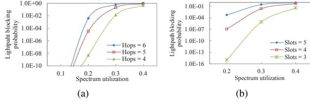
Fig. 2. (a). Lightpath blocking probability under different lightpath hops (without spectrum conversion). Number of spectrum slots per lightpath connection = 3; (b). Lightpath blocking probability under different number of required slots (without spectrum conversion). Number of lightpath hops = 3.
