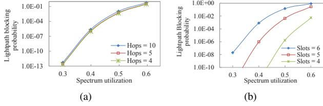
Fig. 1. (a) Lightpath blocking probability under different lightpath hops (with spectrum conversion). Number of spectrum slots per lightpath connection = 5; (b) Lightpath blocking probability under different numbers of required spectrum slots (with spectrum conversion). Number of lightpath hops = 4;
