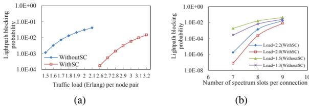
Fig. 3. (a) Lightpath blocking probability under different lightpath hops (with spectrum conversion). Number of spectrum slots per lightpath connection = 5; (b) Lightpath blocking probability under different numbers of required spectrum slots (with spectrum conversion). Number of lightpath hops = 4;
